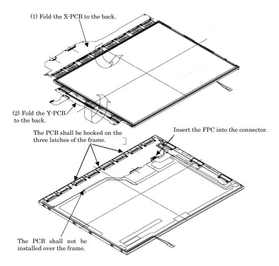
Figure 4-58 Replacing TMD fluorescent lamp (WXGA) (8)
